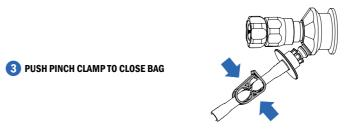
Engage the pinch clamp to seal the Keofitt Sterile Sampling Bag.
