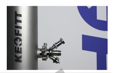
12. Install the valve head in its "open" position. Make sure to only fasten the head as little as possible, still securing though, the head is firmly fixed to the valve body. This is done by turning the hex nut approximately 360 degrees or only until the valve body's thread becomes invisible. By doing this, it will leave enough free space inside the valve body to allow for the Emergency Tool to pass the membrane when dismounting the Emergency Tool.
