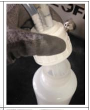
Connect the lower port, pushing the toothed jaw onto the fitting, and sliding the flanged connector over the top to secure in place. Attached the lower, which will support the bottle, then the upper in the same fashion.
